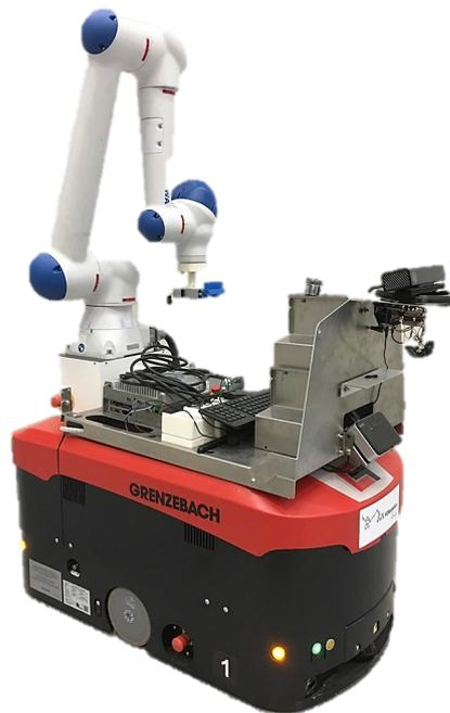
Imagine that your employer is **planning to implement a new robot**. As in the figure, this is an automated vehicle with a robot arm (manipulator) that allows the robot to perform tasks such as bin picking or assembly work. For example, it can pick up and transport individual products or assembly parts from the warehouse or assist with assembly tasks. Furthermore, this robot can move independently through the work area and is able to communicate and cooperate with humans.
